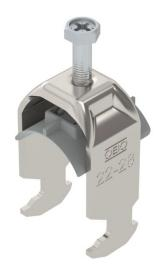
Clamp clip with hammerhead foot, plastic pressure sleeve made of polypropylene. For vertical and horizontal mounting of 1 single cable on a C-profile rail. For a slot width 16–17 mm. With 1-start screw thread on pressure sleeve, universal hexagonal screw head WAF10, with slot and cross recess. Suitable for assembly indoors and outdoors. We recommend the use of a counter-sleeve.
