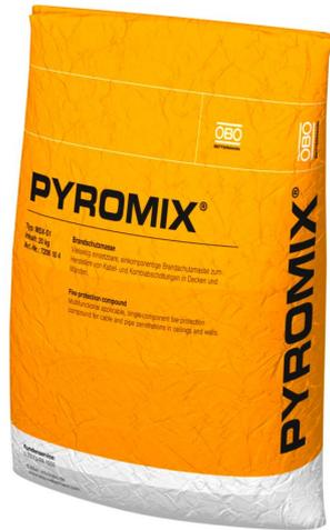
Mortar to create cable and combination insulation in solid walls and ceilings. Suitable for pumping, pressing and for manual installation. Adding approx. 6 litres of water to 20 kg of dry mortar produces about 20 litres of workable compound. For interior application.
