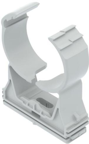
Highly stressable clip for accepting plastic or metal electrical and sanitary pipes as well as the electrical installation pipe Quick pipe. Universal fastening options on walls, ceilings and steel constructions, both indoors and outdoors. Flexible clamping range of several millimetres. Toolless pipe mounting. Connectable to each other to Ø 32 mm, also with the OBO Quick or Multi Quick clip. For variable distances and clip quantity mountable on a profile rail.
