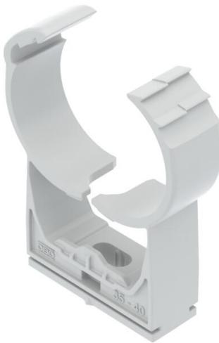
Highly stressable clip for accepting plastic or metal electrical and sanitary pipes as well as the electrical installation pipe Quick pipe. Universal fastening options on walls, ceilings and steel constructions, both indoors and outdoors. Flexible clamping range of several millimetres. Toolless pipe mounting. Connectable to each other to Ø 32 mm, also with the OBO Quick or Multi Quick clip. For variable distances and clip quantity mountable on a profile rail.
