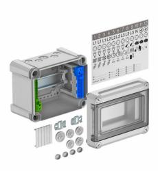
Distribution box with terminal strip for surface mounting, for the current sub-distribution in interior and exterior areas, in accordance with IEC 439-3. With premounted 35 mm hat profile rail. IP66 protection type and IK08 protection rating. Transparent cover to screw on, with cut-out.
