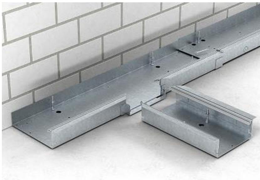
Should the **OKB-U..ON** trunking need to be connected with the **OKB-E..ON** infeed trunking, then T pieces must be installed and fastened at the appropriate places in the trunking section. Adjust the required system height and secure it with a locknut.
