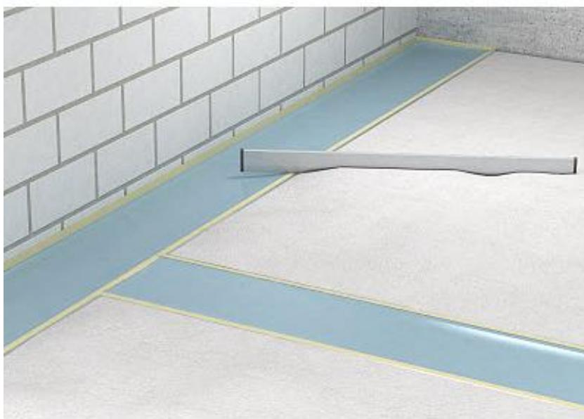
The screed should be installed directly after the OKB trunking system. If necessary, trunking joints must be sealed. The screed layer should line the side profiles and to work the screed carefully and cleanly. A separating layer of 3–5 mm is permitted, but must end below the support profile.
